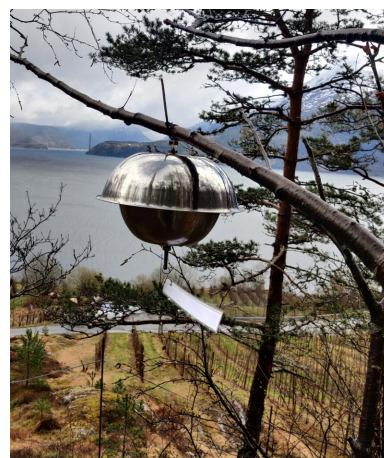
Passive sampling with PUF through the growth season (ca. 3 months) along transects through the orchards in the 4 locations.
