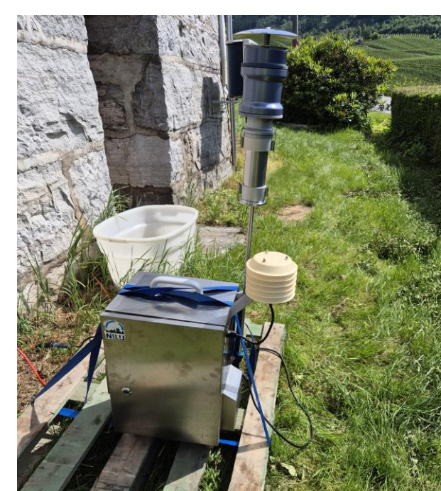
Active air sampling for 1 week-long periods every month during the growth season to get the general background concentrations.
