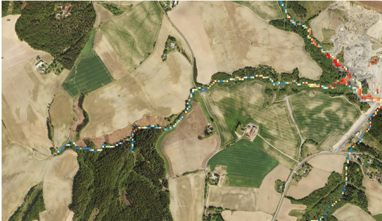
Fig. 4.5. First ranking of locations for constructed wetlands, combining contributing area and location slope.
