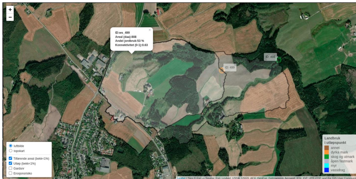
Fig. 4.8. Section of an interactive map displaying two potential locations for constructed wetlands. In this example, the suitability parameters (text box in the centre) are hydrological connectivity and the percentage of agricultural land use in the contributing area.
