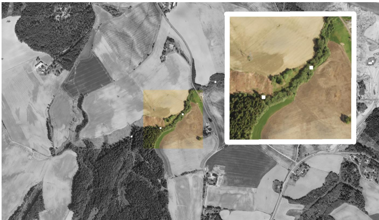
Fig. 4.6. Reducing the number of locations of Fig. 4.5 (50 m or more along the profile, slope inclinations of 1% or less).
