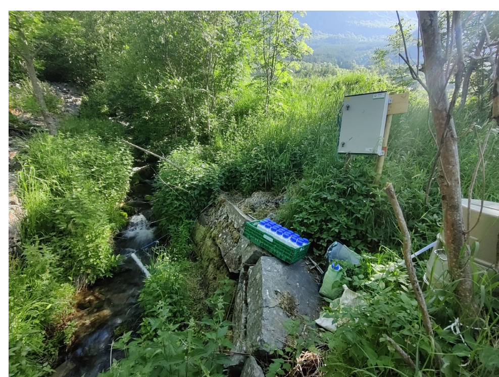
Daily water samples were taken from two small streams running through the orchards. Sampling was done daily with an ISCO sampler, but weekly mixed samples were analyzed. Sampling was done from April to October/November over two years.
