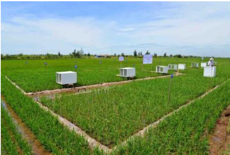
Nam Dinh, Vietnam: Measuring GHG emissions in rice fields. Photo: Trond Rafoss
