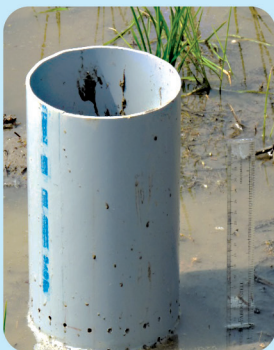
Safe AWD = Irrigate when water depth ~ 15 cm
